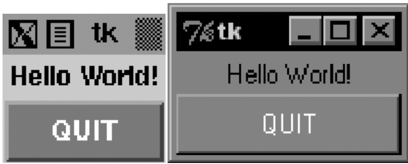
图 19-3 Tkinter Label and Button widgets (tkhello3.py)
