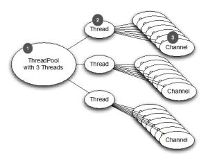
Figure 15.6 Thread allocation for nonblocking transports (such as NIO and AIO)
