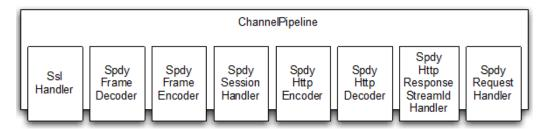
Figure 12.3 ChannelPipeline if SPDY is supported
