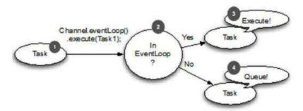
Figure 15.5 EventLoop execution logic / flow
