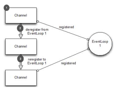
Figure 16.2 Deregister and reregister with an EventLoop
