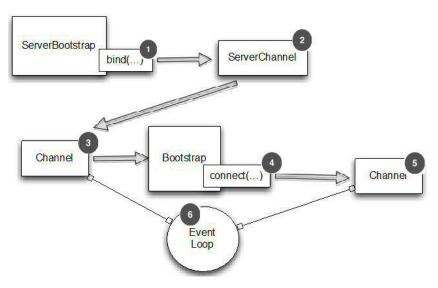
Figure 9.4 Share EventLoop between channels with ServerBootstrap and Bootstrap
