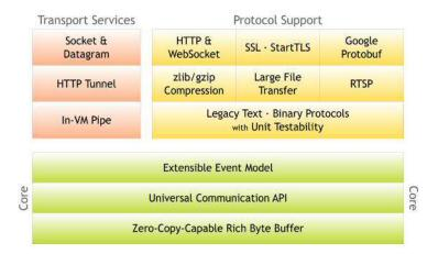
Figure 1.1 Overview of the model, transports, and protocols
