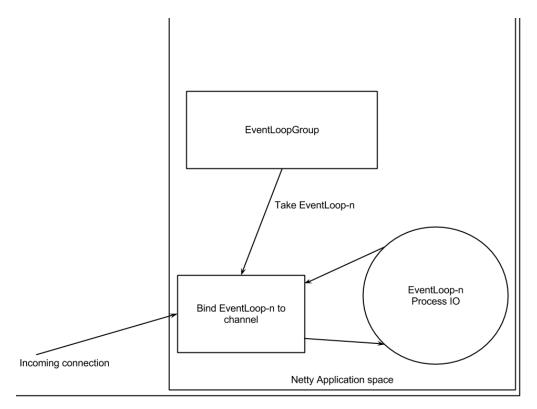
Figure 3.1 - Diagram showing an EventLoopGroup and a Channel being bound to a single EventLoop permanently
