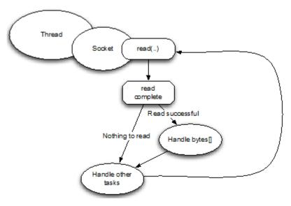
Figure 4.3 OIO-Processing logic
